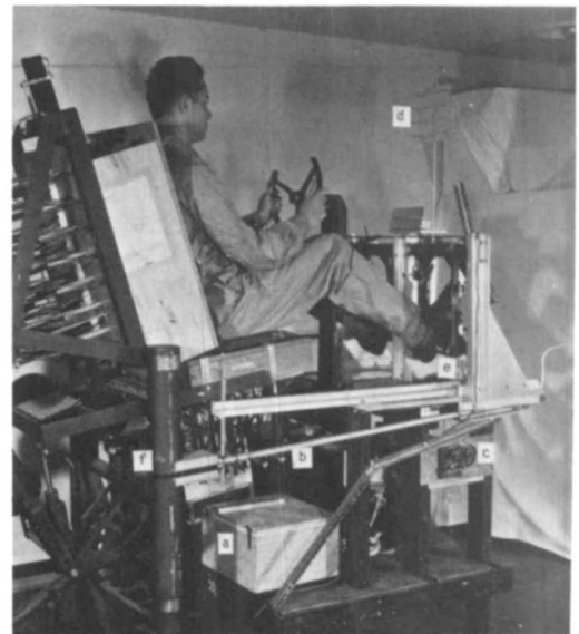
Figure 2. General view of equipment: (a) sound-proof box for inverter; (b) rudder-bar adjustment rod; (c) torque-indicator dial; (d) eye-level indicator; (e) heel-marking tape; (f) screw-jacks.
