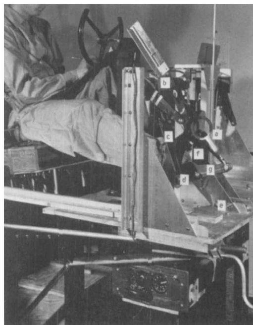
Figure 3. View of pedal and strain-gauge equipment: (a) stress-ring; (b) angle-iron bracket; (c) hanger; (d) rudder bar; (e) rudder-bar lock; (f) brake pedal; (g) lever.
